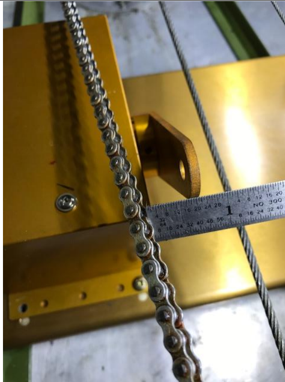
IMAGE 7-2 PITCH SERVO ARM ALIGNMENT
