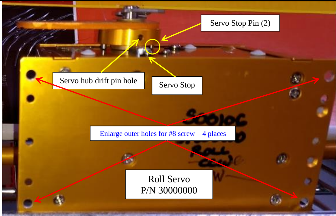
IMAGE 3-9 ROLL SERVO HUB DRIFT PIN AND LOCKING PIN HOLE ALIGNMENT
