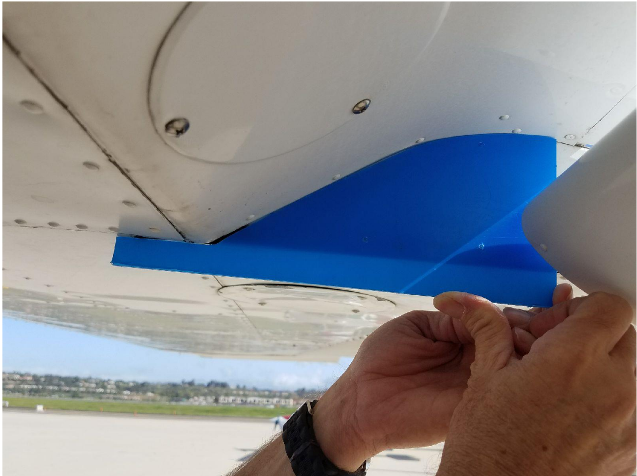
IMAGE 3-4 DRILL TEMPLATE MOUNTED AT WING STATION 100.5
