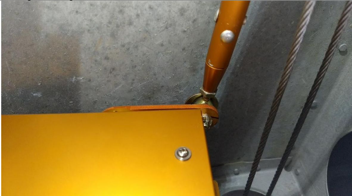
IMAGE 3-10 ROLL SERVO PUSH PULL TUBE ASSEMBLY
