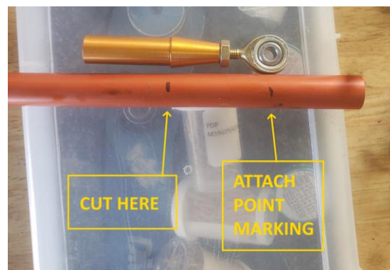
IMAGE 3-11 TRIMMING PUSH PULL TUBE
