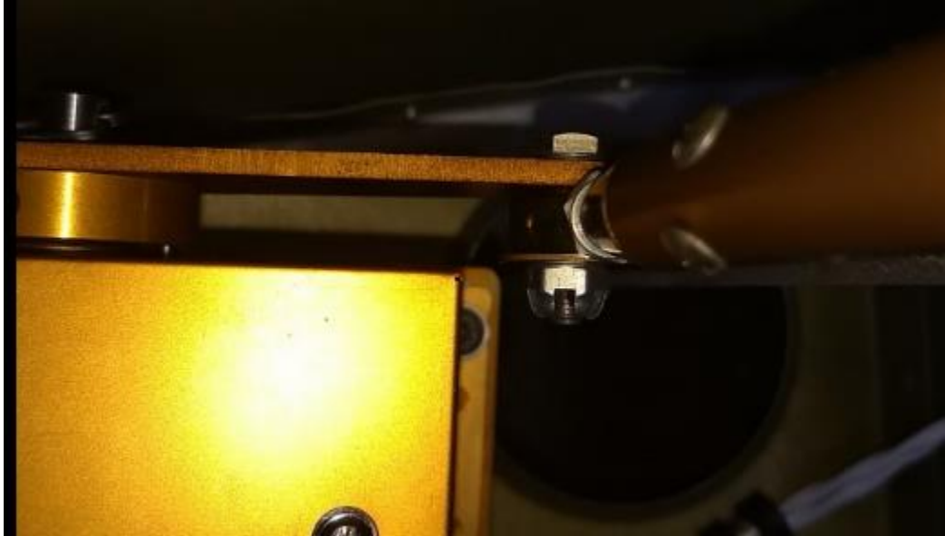
FIGURE 3-11 ROLL SERVO PUSH PULL TUBE ASSEMBLY
