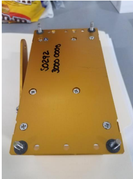
FIGURE 3-9 10085 RETAINERS AFFIXED TO MS27038-0807 SCREWS
