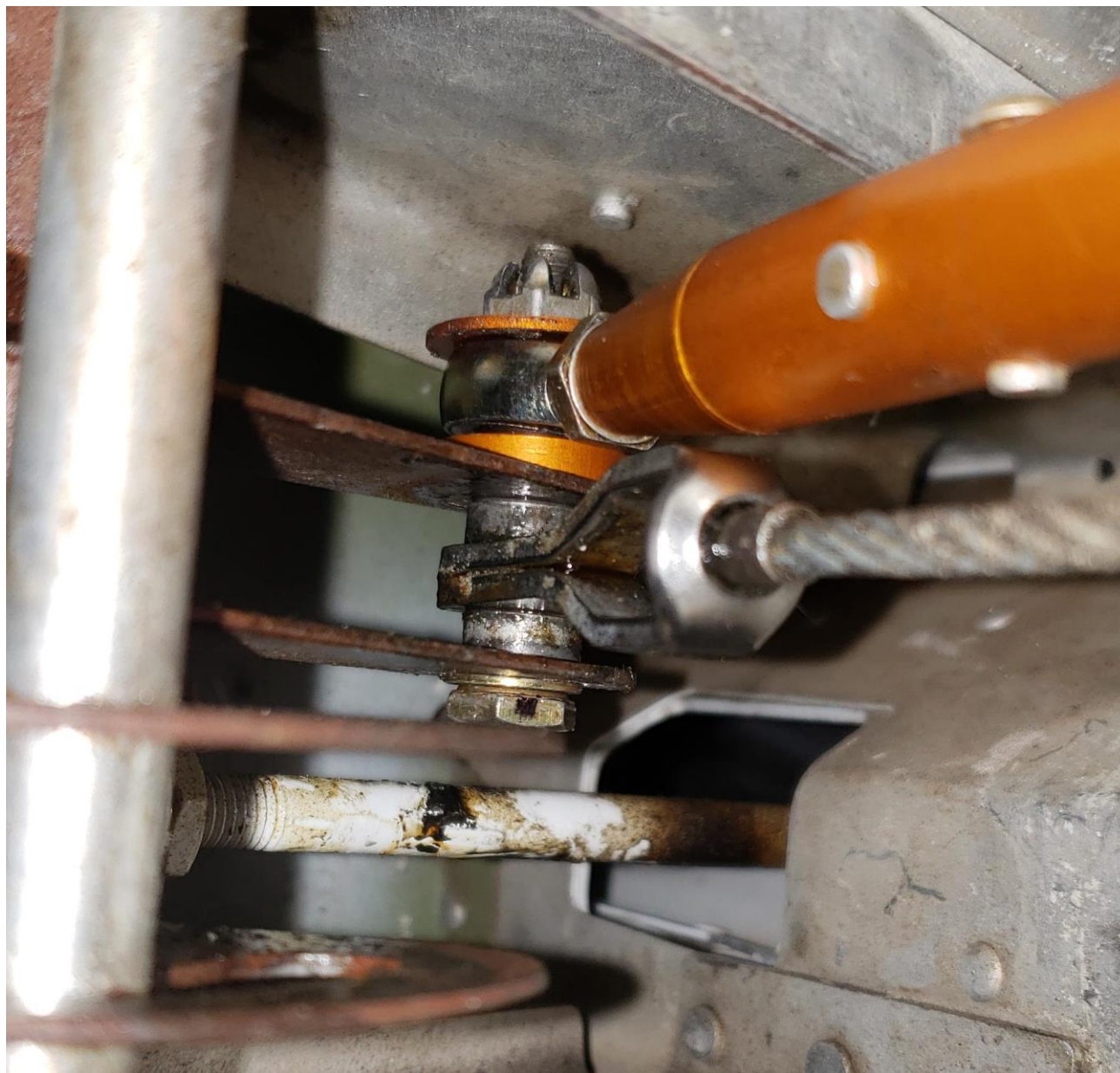
D- 7 ROLL PUSH PULL TUBE BELLCRANK HARDWARE STACKUP
