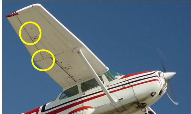
FIGURE 3-1 WING ACCESS COVER LOCATIONS
