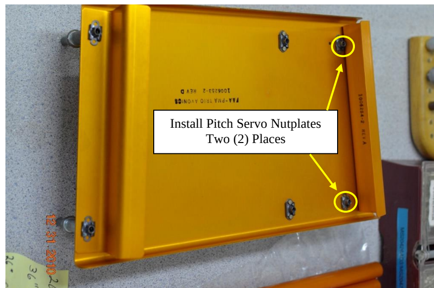
FIGURE 4-5 PITCH SERVO NUPLATE INSTALLATION
