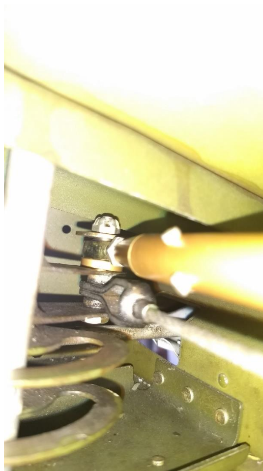
FIGURE 3-16 AILERON BELLCRANK INSTALLATION
