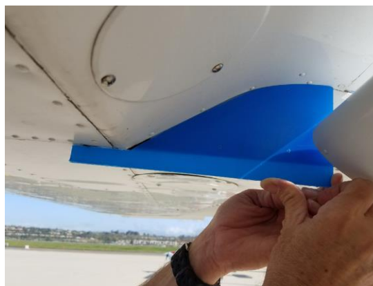
FIGURE 3-3 DRILL TEMPLATE MOUNTED AT WING STATION 100.5
