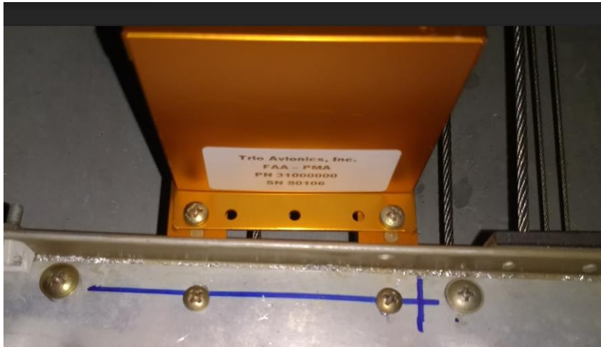
FIGURE 3-12 LH & RH ANGLES FASTENED TO ACCESSORY TRAY
