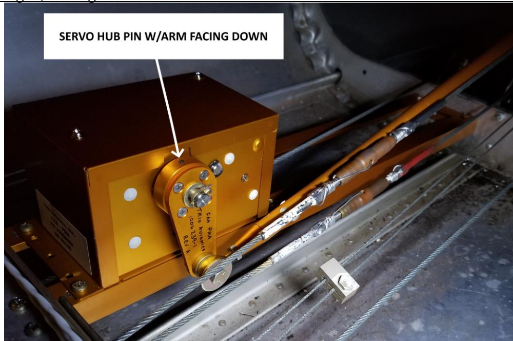
FIGURE 3-13 SERVO HUB PIN & ARM ALIGNMENT
