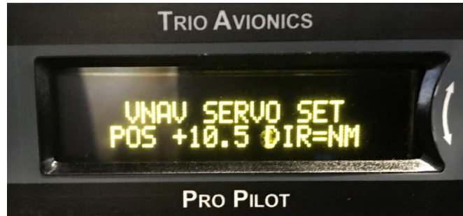
IMAGE 4-11 ELEVATOR POSITIONED IN NEUTRAL (EXAMPLE)
