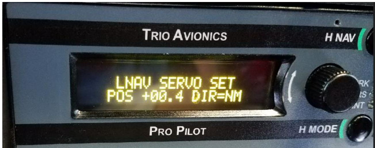
IMAGE 3-11 LNAV SERVO SET SHOWING SERVO ARM POSITION
