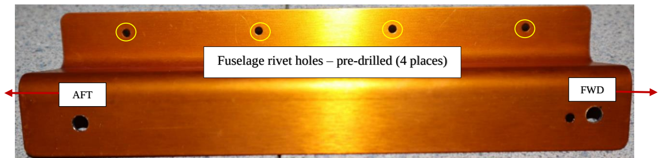
IMAGE 4-4 ZEE ANGLE MATCHED DRILLED FOR SERVO SCREWS
