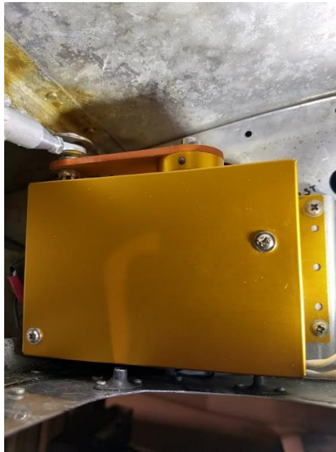
FIGURE 3-8 ROLL SERVO INSTALLATION
