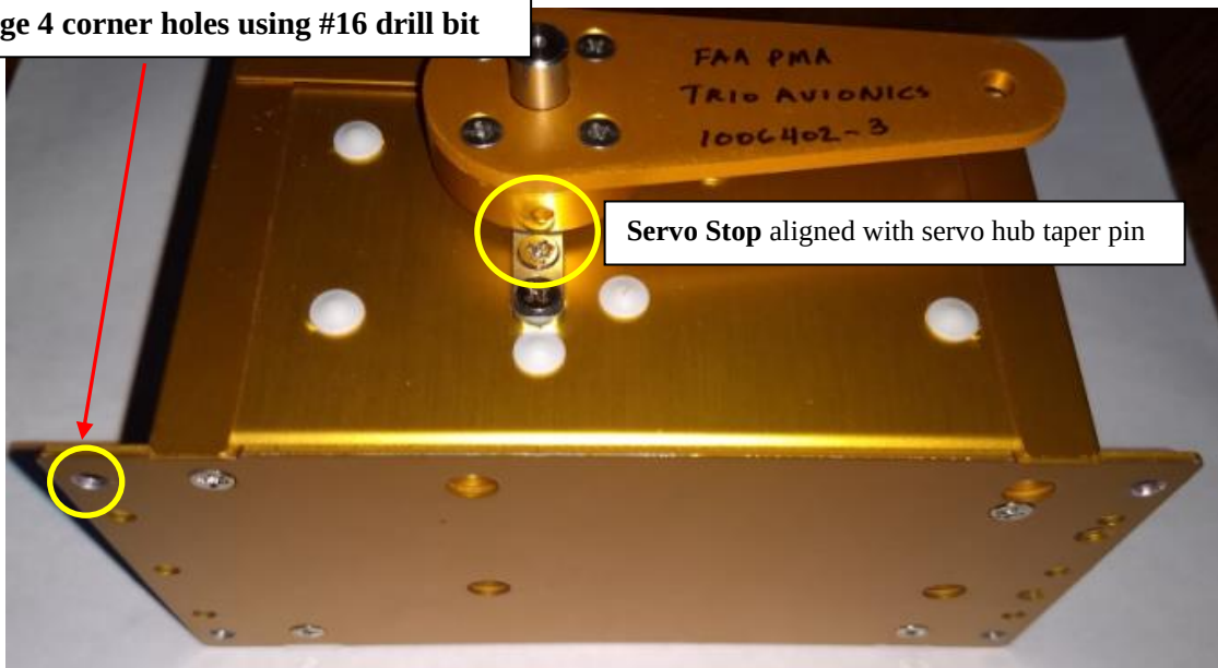
FIGURE 3-7 ROLL SERVO HUB DRIFT PIN / LOCKING PIN ALIGNMENT
