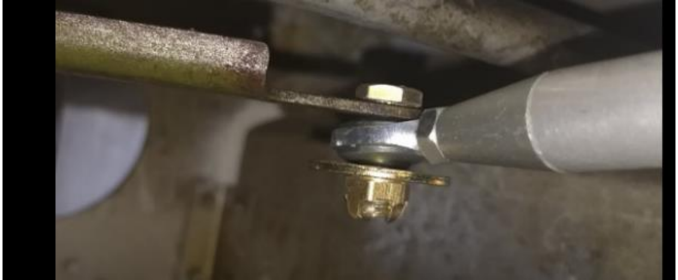
FIGURE 3-11 PUSH PULL TUBE ATTACHMENT AT AILERON BELLCRANK
