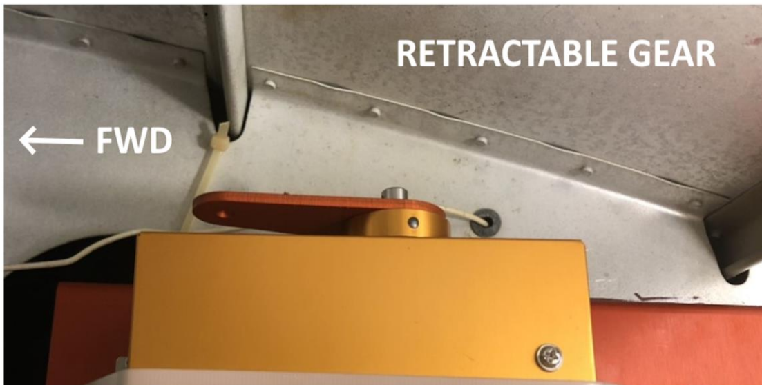
FIGURE 4-8 COMMON ROLL SERVO INSTALLATION (EXPLODED VIEW)
