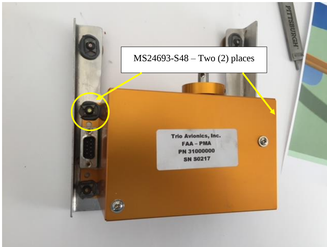
IMAGE 3-3 ROLL SERVO BRACKET INSTALLATION
