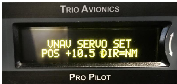
IMAGE 5-3 ELEVATOR POSITIONED IN NEUTRAL (EXAMPLE)
