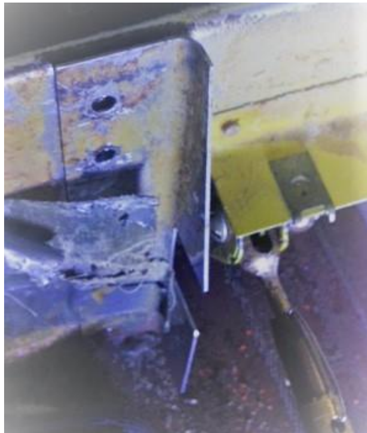
IMAGE 3-1 ANGLE STIFFENER AND AILERON (ROLL) CONTROL HORN
