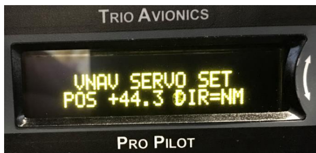
IMAGE 5-5 ELEVATOR FULL DOWN
