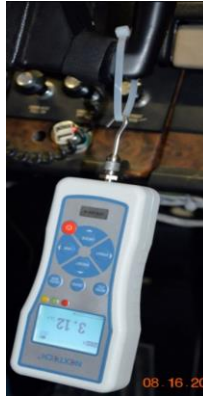
FIGURE 5-2 ROLL SERVO FORCE GAUGE MEASUREMENT (NEXTECH DFS500 FORCE GAUGE SHOWN)
